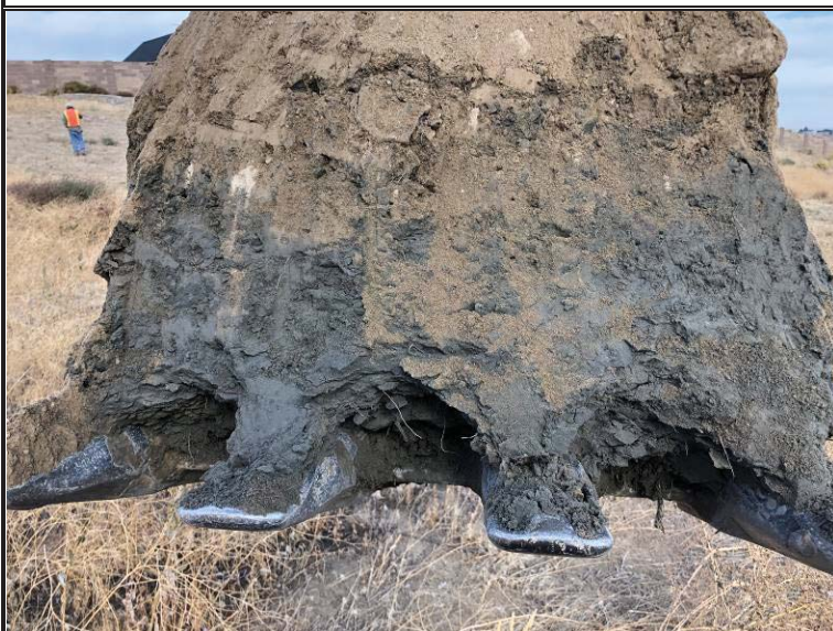
Gray-colored organic-rich apparent native silts in test-pit TP-4
