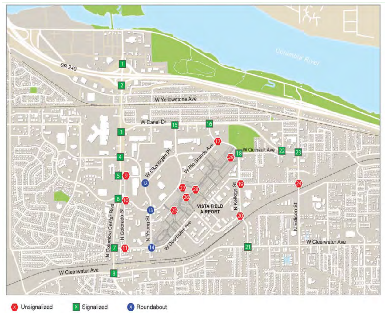
Transportation System Impact Evaluation Intersections Off-Site
