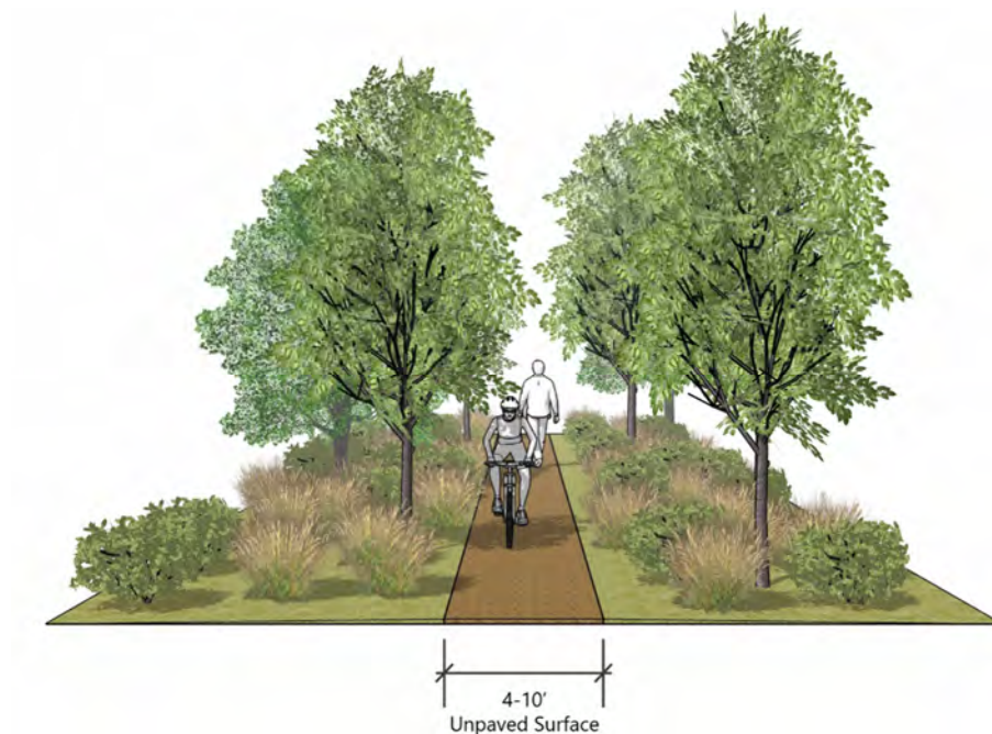
Figure 5. Natural Trail Typical Cross-Section
